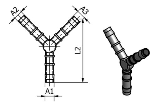
Ext. Hose Diameter A1 = 5 Ext. Hose Diameter A2 = 5 Ext. Hose Diameter A3 = 5 L2 = 43
